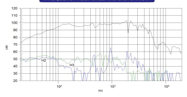
Note: On axis frequency response measured with loudspeaker standing on infinite baffle in anechoic chamber, 2,83V @ 1m
