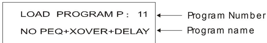
Then, turn CHA to select one program(1-11) . Press CHB button again, save the setting and load the selected program. At the same time, the LCD shows: LOADING .....Several seconds later, the LOADING is finished and the system return the menu
