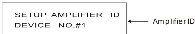
Then, turn CHA to change the amplifier ID from 1 to 255. Press CHA button again and save the setting.
