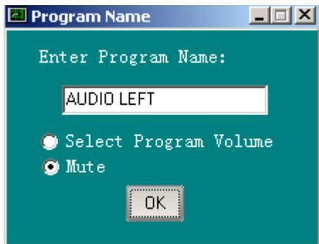
The user can select the file gain in File Down mode (the parameter gain in Setup Down mode) or mute when download the program. Such gain can be effective only if the unit is in the offline mode and AUTO MUTE is OFF. In online mode, the unit will download the file and recall the program when New or Open the file. If the current program is No.21, the user can't New or Open the file.
