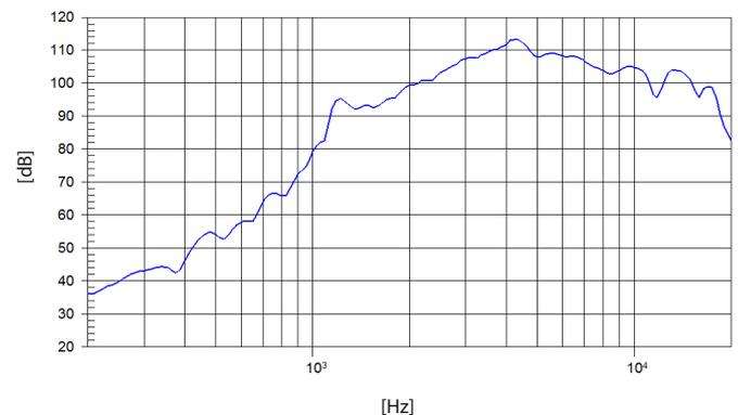
**Note:** On axis frequency response measured coupled to TD-2012/N horn in anechoic chamber, 1W / 1m
